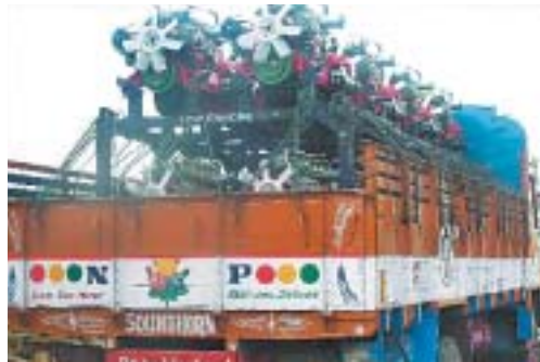
Two-tier stillage: 16 engines per truck.
